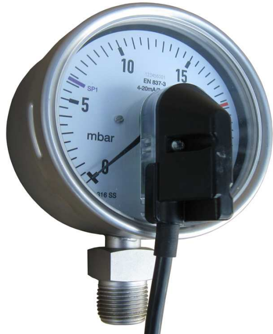
4...20 mA transmitter and 2 contacts (sample: capsule gauge PCX100XA 0 - 25 mbar)
